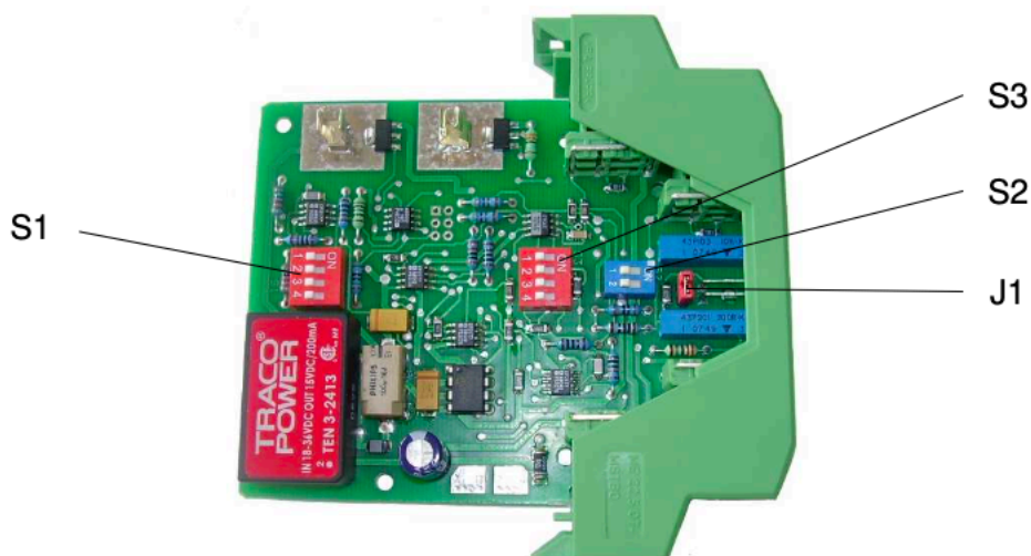
Fig. 2. Location of the jumper and DIP switches on the printed circuit board
