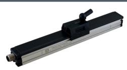
The working principle of ILT-10series inductive linear position sensors depends on the RLC coupling between the positioning element and the sensor. An output signal is provided according to the position of the positioning element. Thanks to the touchless working principle, they are long-lastingsince there are no factors such as wear and tear.
