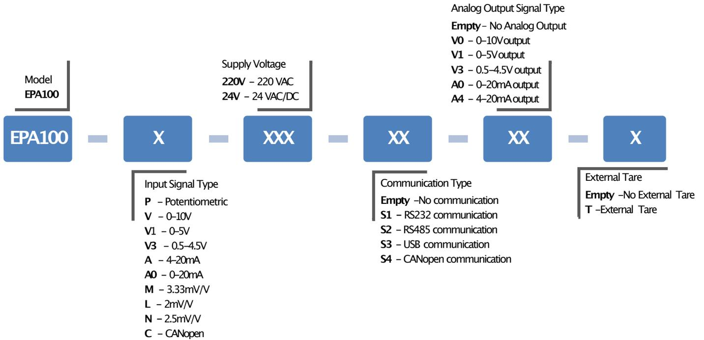
\*If the input signal type is selected as mV/V (M, L, N), the analog output signal (V0, V1, V3, A0, A4) cannot be received.
