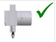
3. If there is a trickle of water (like a rain), the wire outlet must not be a drip of water upstream. If needed please use guide rollers.
