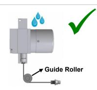
4. The wire should not be pulled in angular. If needed, please use guide rollers.
