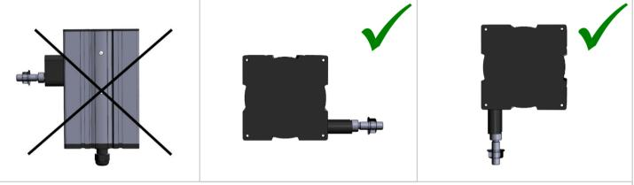
3. If there is a trickle of water (like a rain), the wire outlet must not be a drip of water upstream. If needed please use guide rollers.
