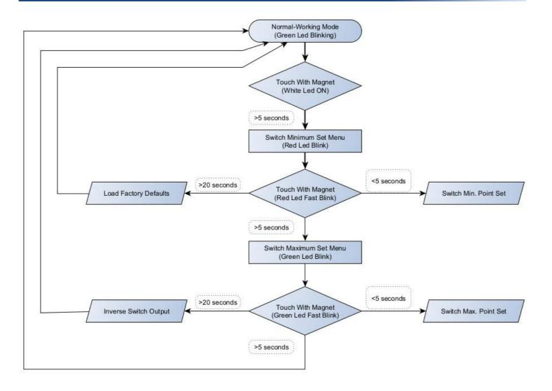
In this menu, the minimum and maximum distance range at which the Switch output of the product will be active is determined.
